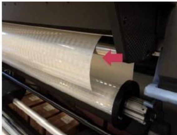
Figure 8. Leading edge of sheeting resting beyond metal curing platform prior to printing.
