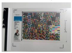
For measuring insert the sample between the two transparent sheets of the sample holder and position inside the corner marks.
