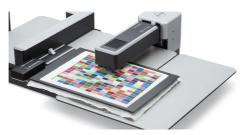
If the material to be fixed is very thin, or elastic, then the chart might only be fixed distorted. In this case use the automatic target recognition option available with the "Textile edition" of the instrument in order for the software to detect correctly the center of the patches,
