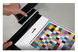
When inserting a new holder, make sure it is inserted until a click noise indicates the final and correct fixing of the sample holder.
