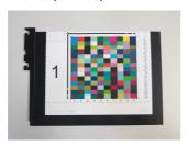
This sample holder allows frame mounting og the color charts and assures no UV-cut filtering occurs when measuring.
