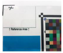
Cut off the reference area of the target to allow the instrument to calibrate to absolute white.
