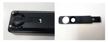
Note: The validity of this reference white is 24 months from the production date. See the serial no. on the reference white. The first four characters indicate the year and the month of production. For example a calibration strip with a serial number B701021indicates: Year: B7=2017, Month: 01= January. This reference white is valid until January, 2019.
