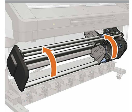
Raise the input-output module to its top position.
