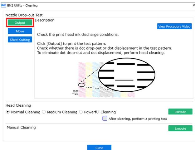
8. Check whether there is dot drop-out or dot displacement in the test pattern.
