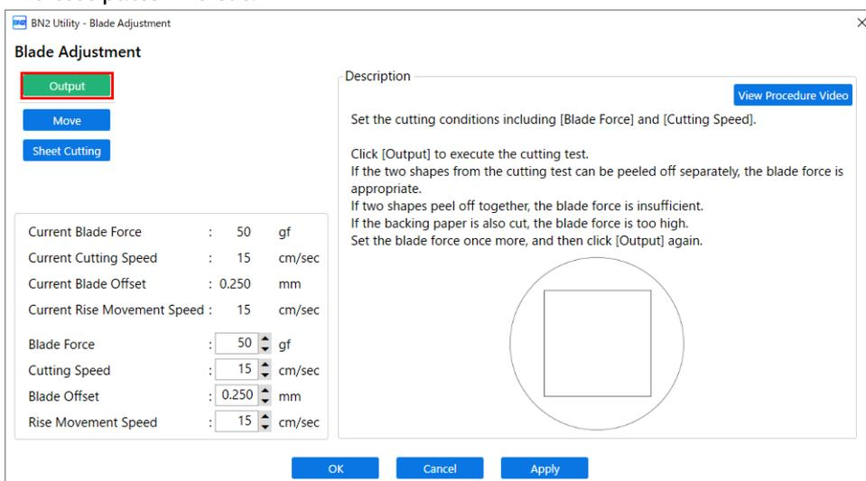
4. Peel off the cut shapes and change the [Blade Force] settings according to the cutting quality.
