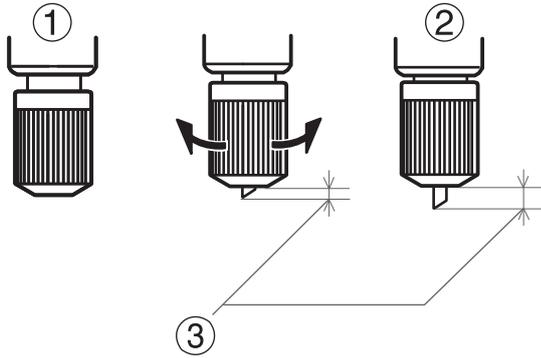
Set the amount of blade extension (③) so that when the cutter pierces the media (④), the blade extends slightly.
