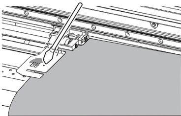
**It may not be possible to detect the media clamps because the multi sensor is dirty with ink due to reasons such as the media striking it immediately after printing.**
