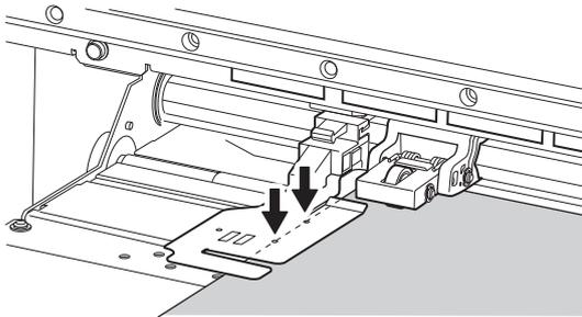
9. Feed the media in the feed direction, checking that the media stays aligned with the pinch rollers.
