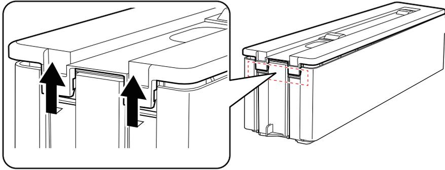
4. Lift up the flap of the drain pack to remove it from the drain cartridge.
