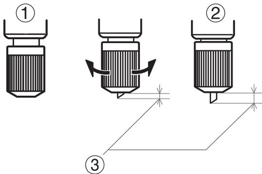
Set the amount of blade extension (①) to an amount that is the sum of the thickness of the media portion (②) and half (④) the thickness of the backing paper (③).
