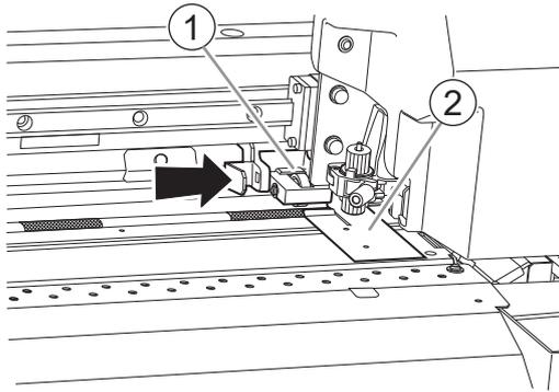
3. Move the left pinch roller (①) and the left media clamp (②) to a position farther left than the media width.
