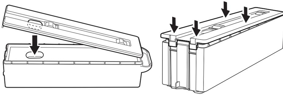
7. Insert the drain cartridge into the machine.
