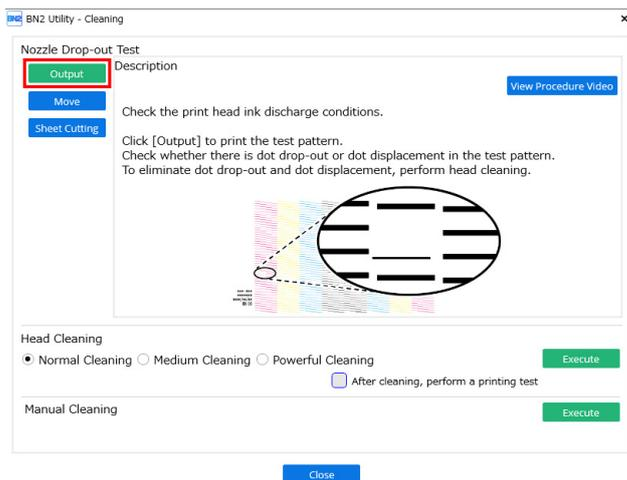
3. Check whether there is dot drop-out or dot displacement in the test pattern.
