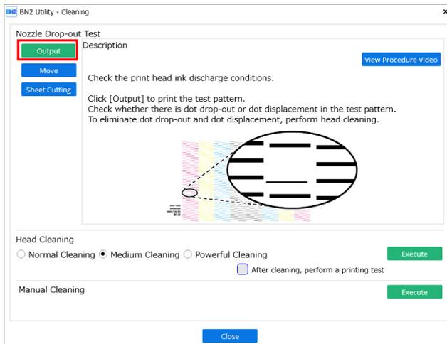
5. Check whether there is dot drop-out or dot displacement in the test pattern.
