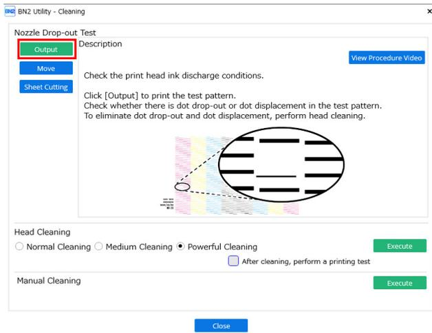
5. Check whether there is dot drop-out or dot displacement in the test pattern. Missing blocks indicate dot drop-out. Collapsed or inclined blocks indicate dot displacement.
