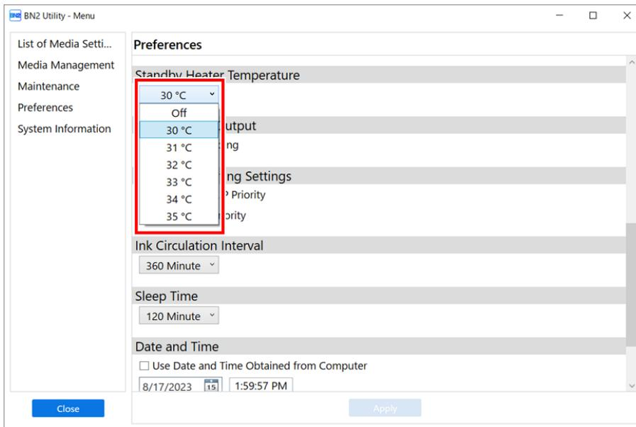
3. Set the heater temperature during standby.
