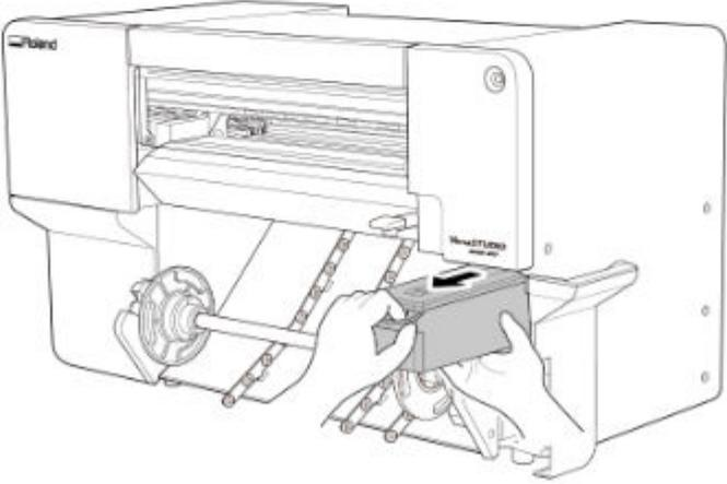
Prepare a replacement drain pack or replace the existing drain pack by following the displayed message.
