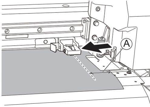
(2) Adjust the right media clamp position as necessary.
