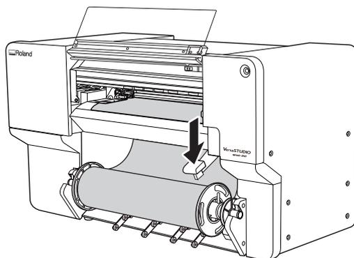
7. Line up the edges of the media with the centers of the holes of the left media clamp.
