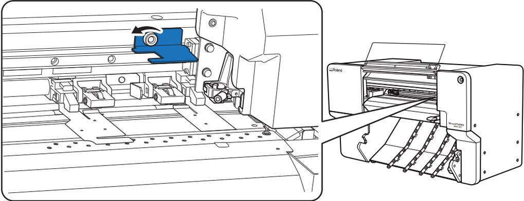
(2) Open the lower-left cover to store the removed retainer and screw.
