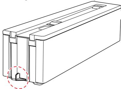
3. Release the hooks in two locations to unlock the drain cartridge lid, and then open it.
