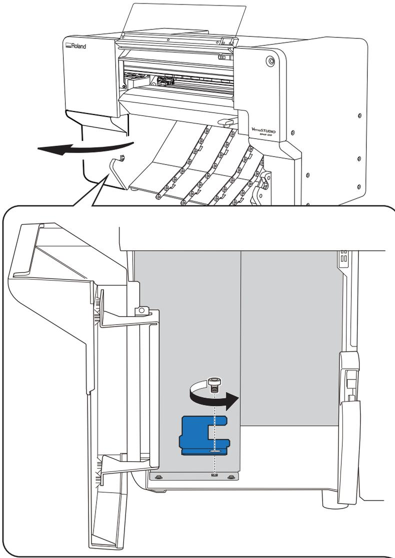
(2) Open the front cover, and then secure the print-head carriage with the retainer.
