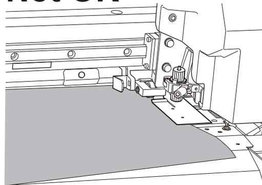
6. Press lightly on the media, and place the left media clamp and left pinch roller on the media.
