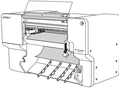
8. Line up the edges of the media with the centers of the holes of the left media clamp.
