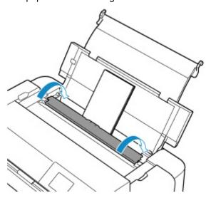
**9.** Select the size and type of envelopes loaded in the top feed at **Page size** and **Type**, select **Register**, then press the **OK** button.
