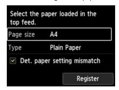
If the loaded paper matches the paper information displayed on the printer's LCD, select **Register** using the  $\triangle \nabla$  buttons and press the printer's **OK** button.
