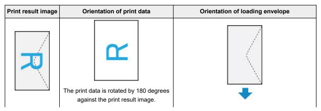
Load the envelope in vertically with the address side facing up so that the folded flap of the envelope will be faced down on the right side.
