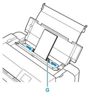
Fold flap of the envelope and load the envelope in portrait orientation with the address side facing up.
