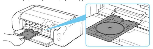
**6.** Insert multi-purpose tray straight in in horizontal direction until arrow (▼) on multi-purpose tray guide is approximately aligned with arrow (△) on multi-purpose tray.
