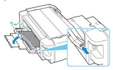
**2.** Slowly pull out paper, either from paper output slot or from manual feed tray, whichever is easier.
