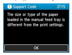
When you press the printer's **OK** button, the paper settings specified when printing are displayed on the LCD.
