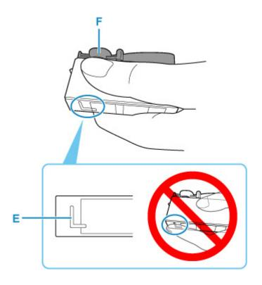
**6.** Twist the orange protective cap (F) 90 degrees horizontally to remove it off GENTLY.
